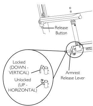
FIGURE 7.3 Removing/Installing Reclining
